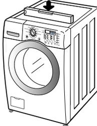
Put an unbalance part (rubber) inside of drum and start QC test mode and run in high spin. (Refer to section 7-2.) When the machine is spinning in high speed, verify that it is stable.
