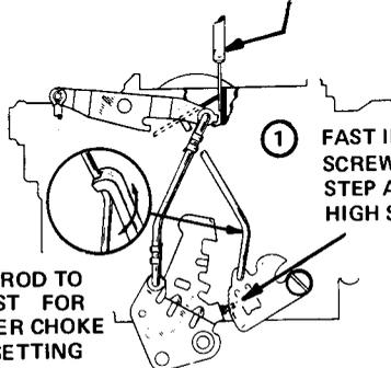
② SPECIFIED GAUGE BETWEEN UPPER EDGE OF CHOKE VALVE AND DIVIDING WALL OF AIR HORN
