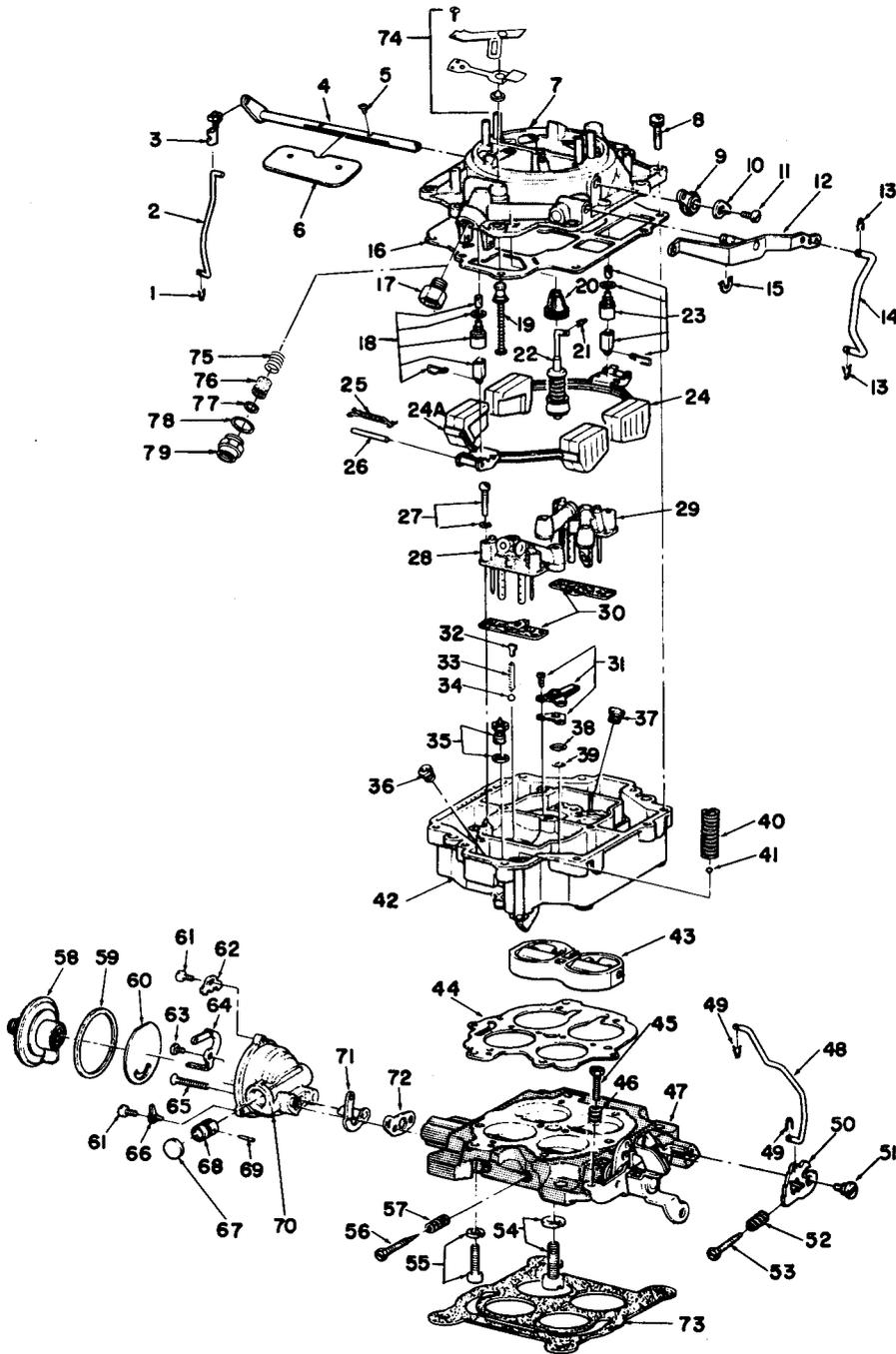
1. Clip—Intermediate Choke Rod (lower)
